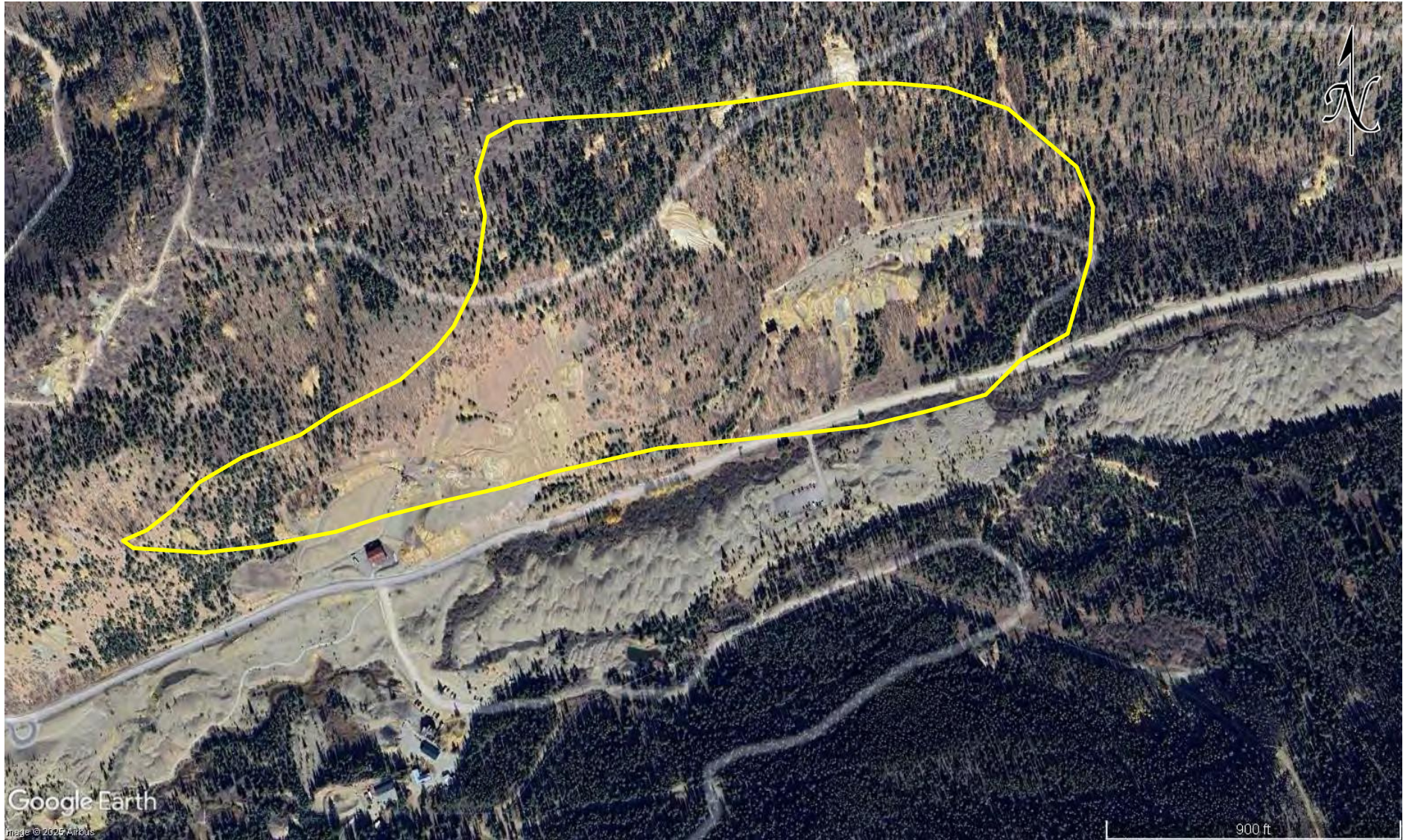
FIGURE 3. APPROXIMATE HORIZONTAL EXTENT OF UNDERGROUND WORKINGS OF THE WELLINGTON-ORO MINE COMPLEX
