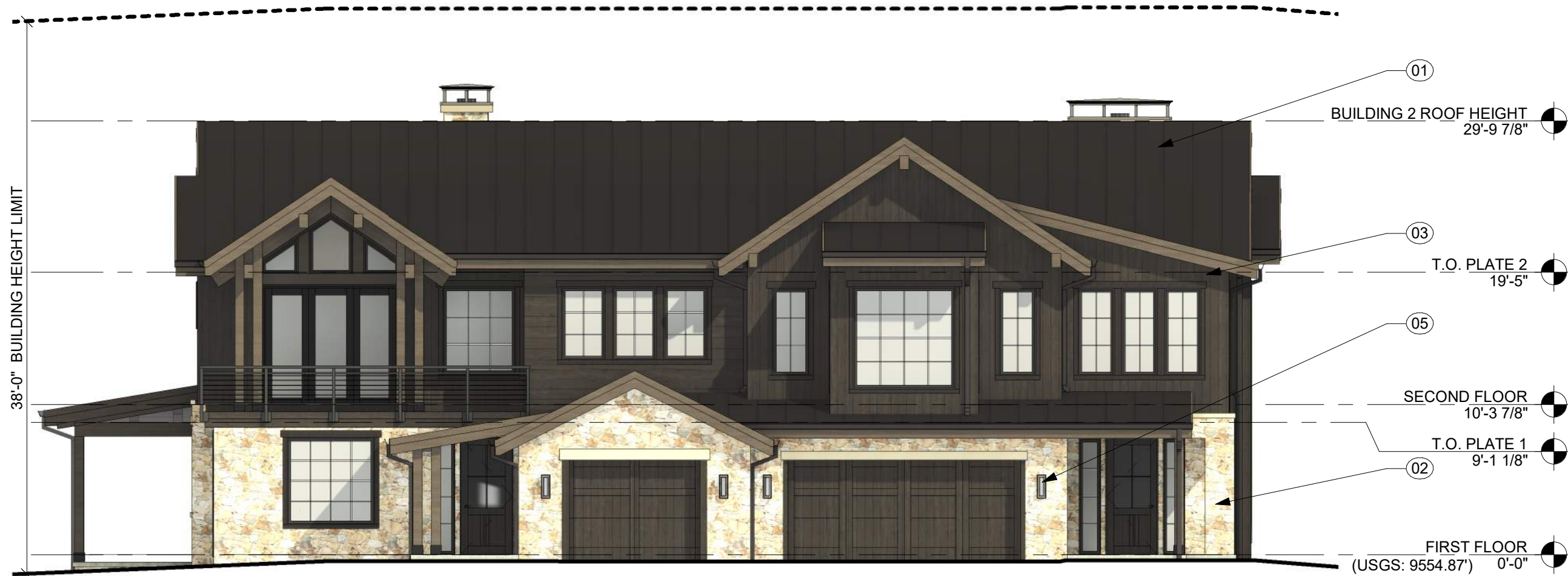
1 BUILDING 2 - FRONT ELEVATION - SCHEME 2 A203 SCALE: 1/8" = 1'-0"
