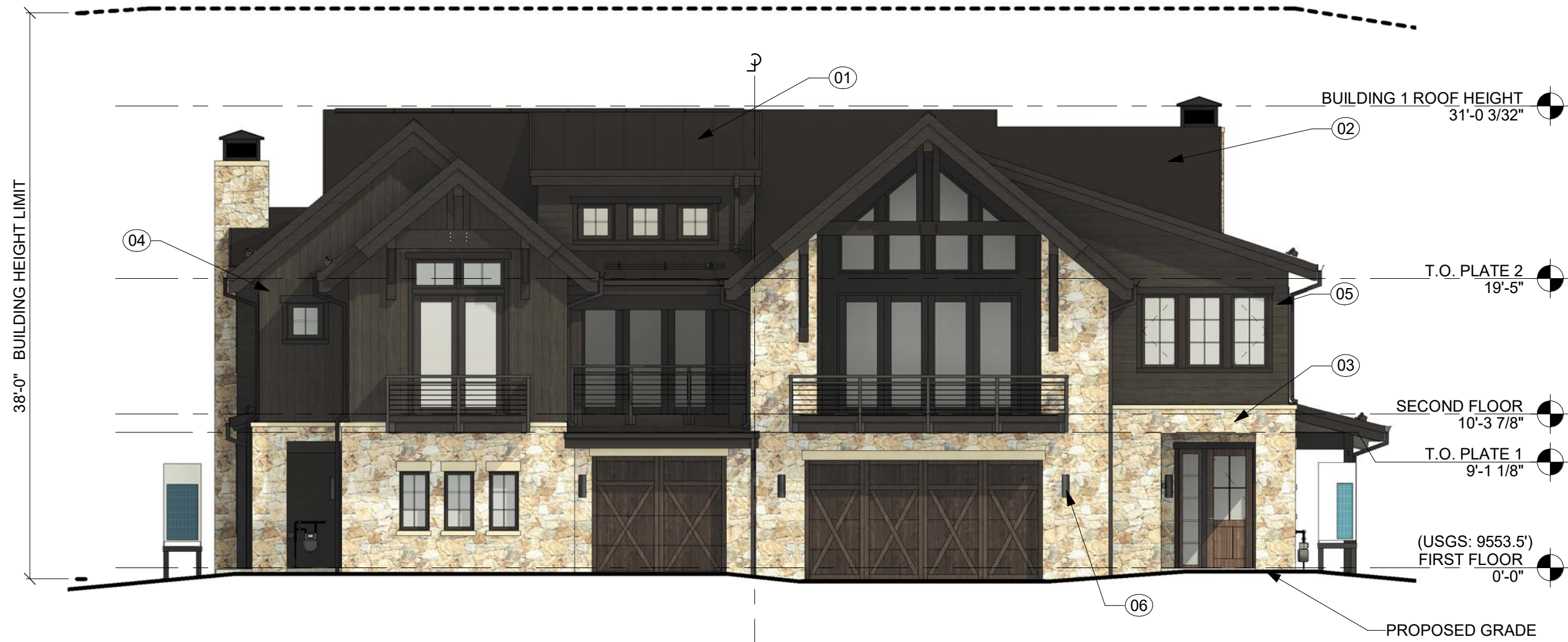
1 BUILDING 1.2 - FRONT ELEVATION - SCHEME 2 A201 SCALE: 1/8" = 1'-0"
