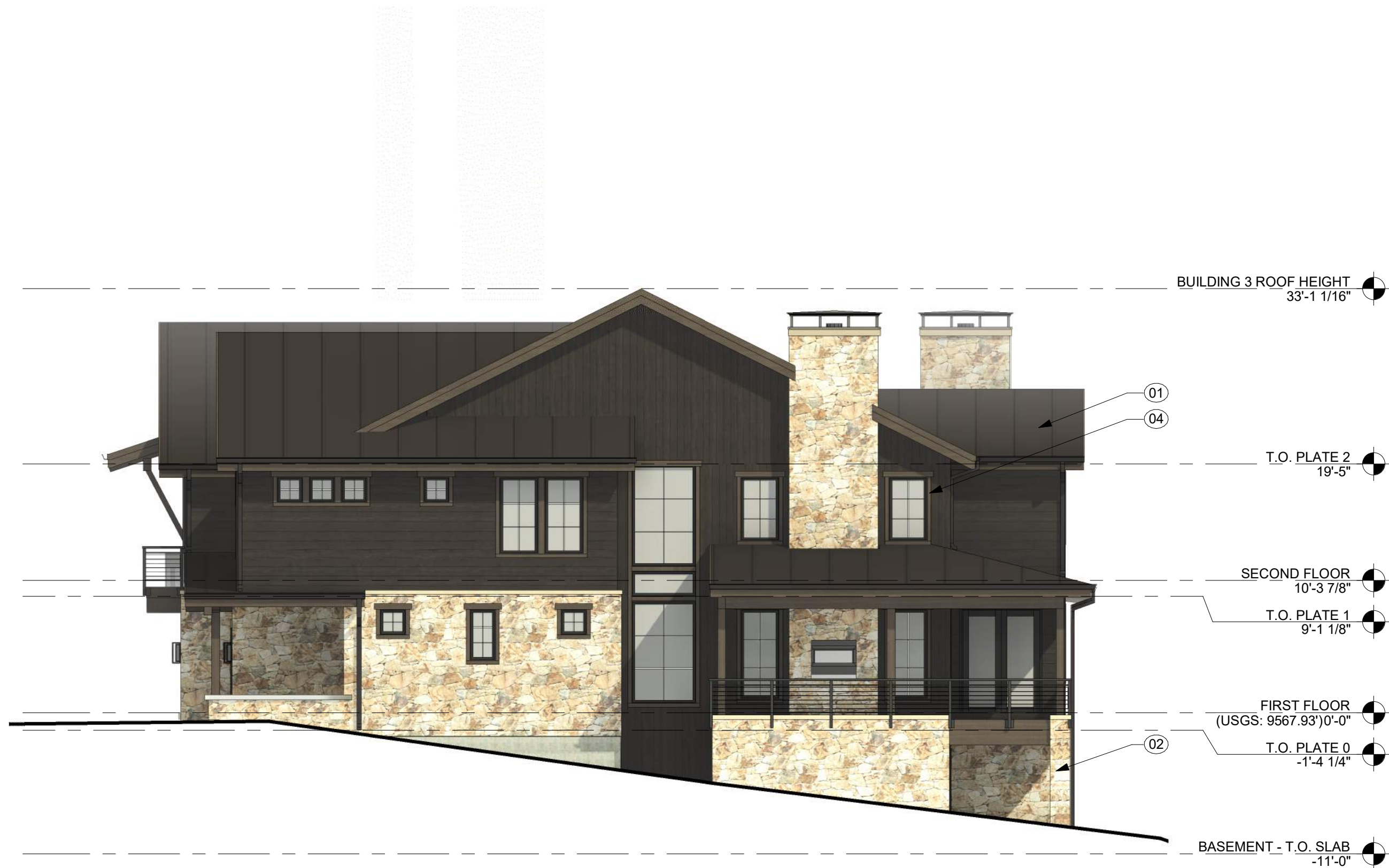
3 BUILDING 3 - RIGHT ELEVATION - SCHEME 2 A206 SCALE: 1/8" = 1'-0"
