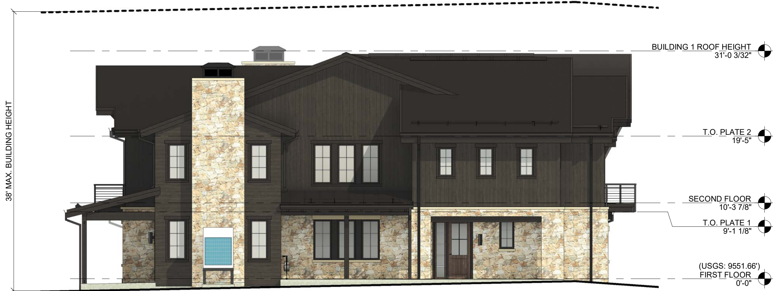
4 BUILDING 1.2 - LEFT ELEVATION - SCHEME 2 A201 SCALE: 1/8" = 1'-0"
