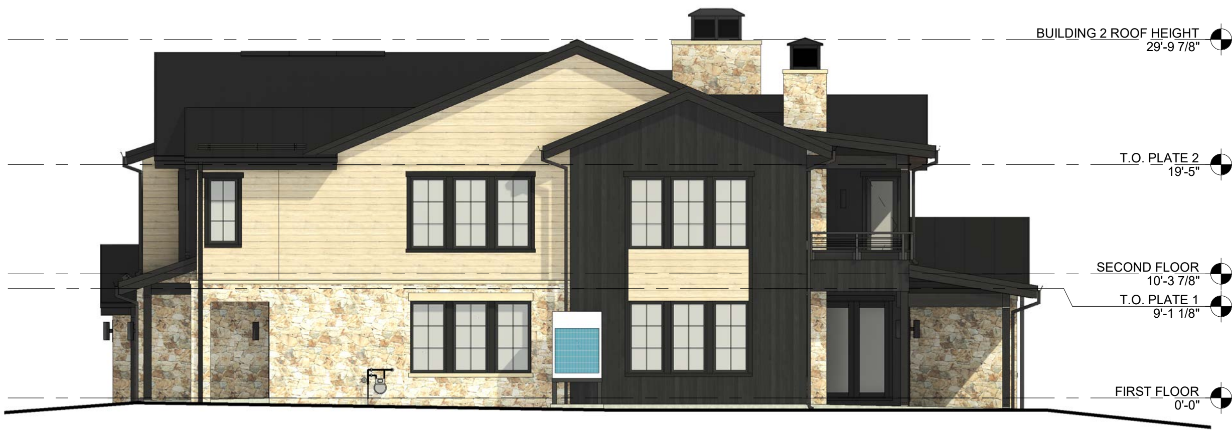
3 BUILDING 2.2 - RIGHT ELEVATION - SCHEME 3 A203 SCALE: 1/8" = 1'-0"
