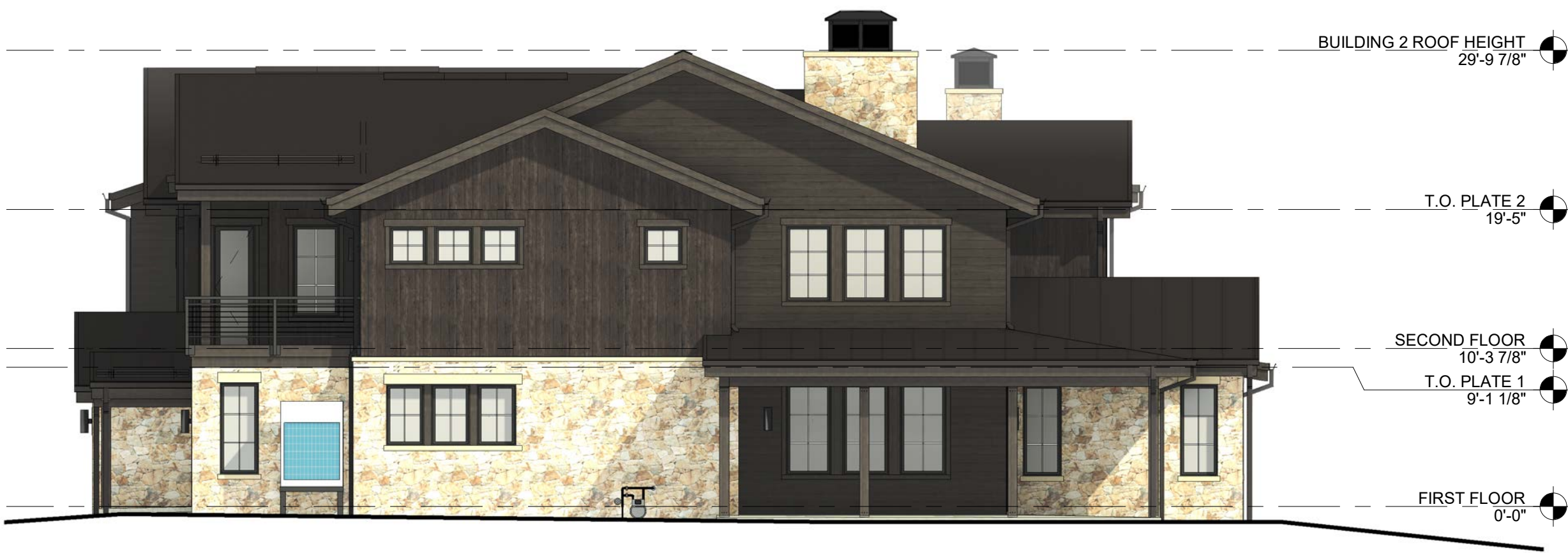
3 BUILDING 2.1 - RIGHT ELEVATION - SCHEME 2 A202 SCALE: 1/8" = 1'-0"
