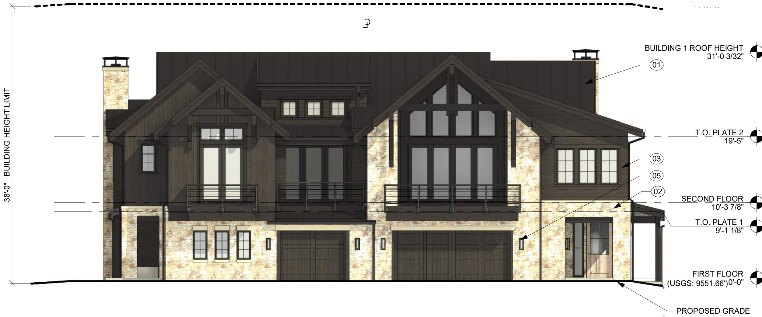
1 BUILDING 1 - FRONT ELEVATION - SCHEME 2 A201 SCALE: 1/8\" = 1'-0"
