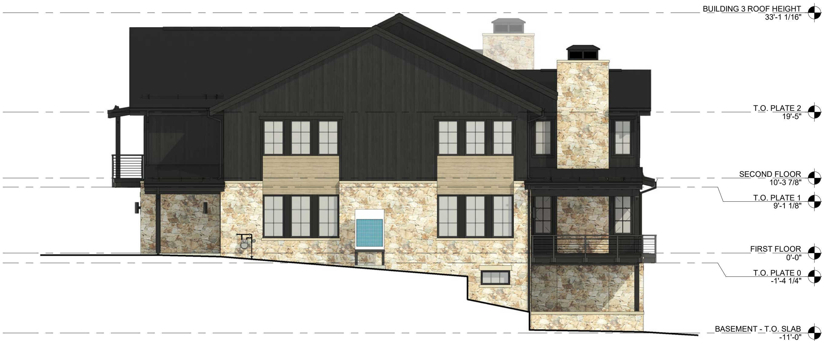
3 BUILDING 3.1 - RIGHT ELEVATION - SCHEME 3 A205 SCALE: 1/8" = 1'-0"
