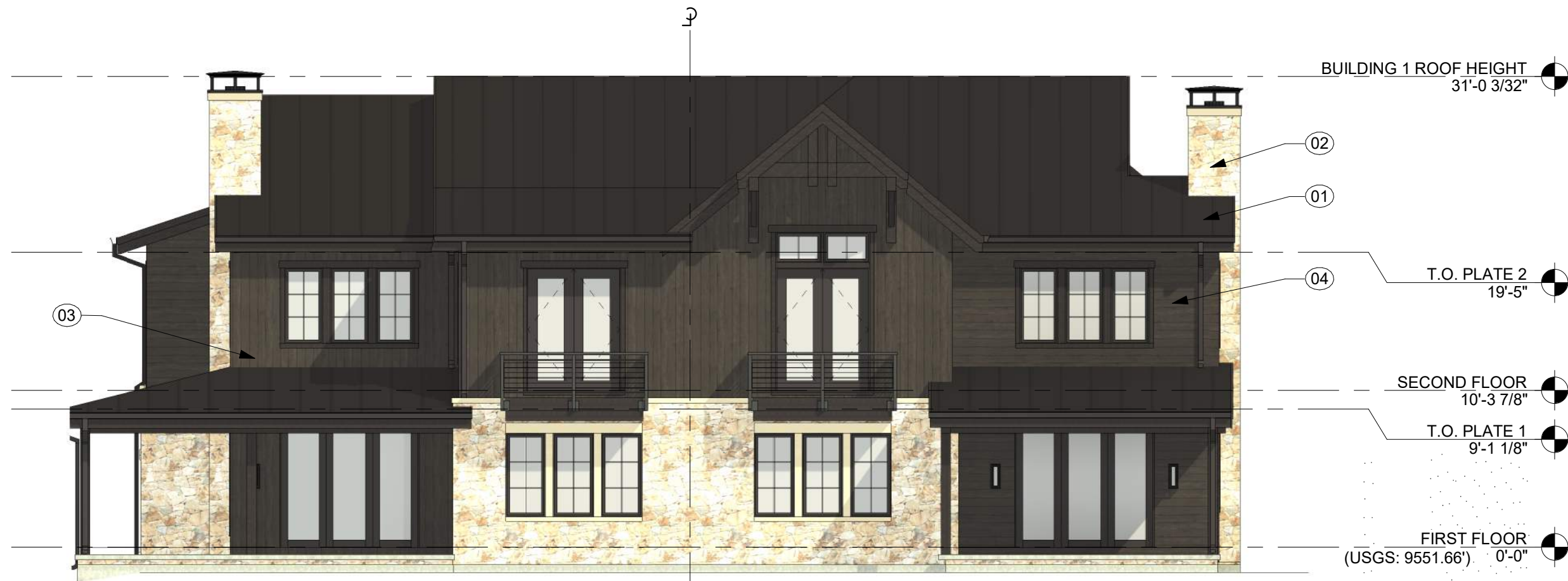
2 BUILDING 1 - REAR ELEVATION - SCHEME 2 A201 SCALE: 1/8\" = 1'-0"
