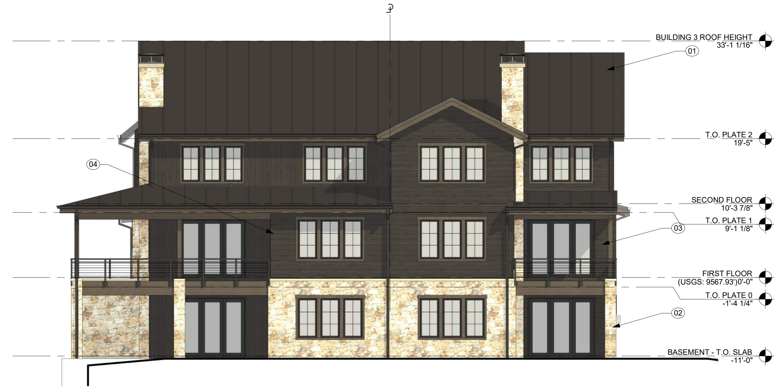
2 BUILDING 3 - REAR ELEVATION - SCHEME 2 A206 SCALE: 1/8" = 1'-0"
