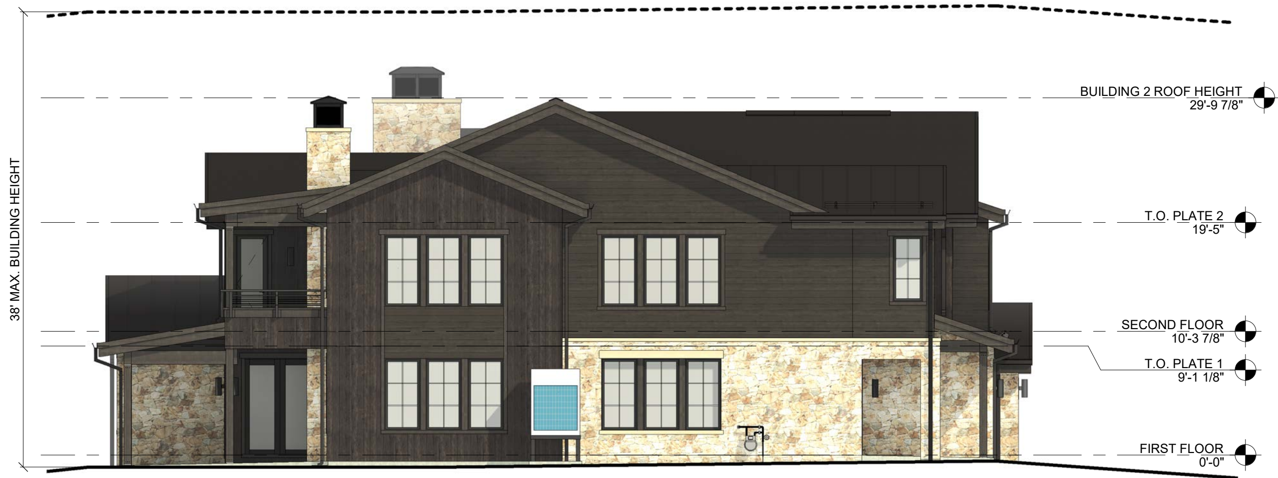
4 BUILDING 2.1 - LEFT ELEVATION - SCHEME 2 A202 SCALE: 1/8" = 1'-0"
