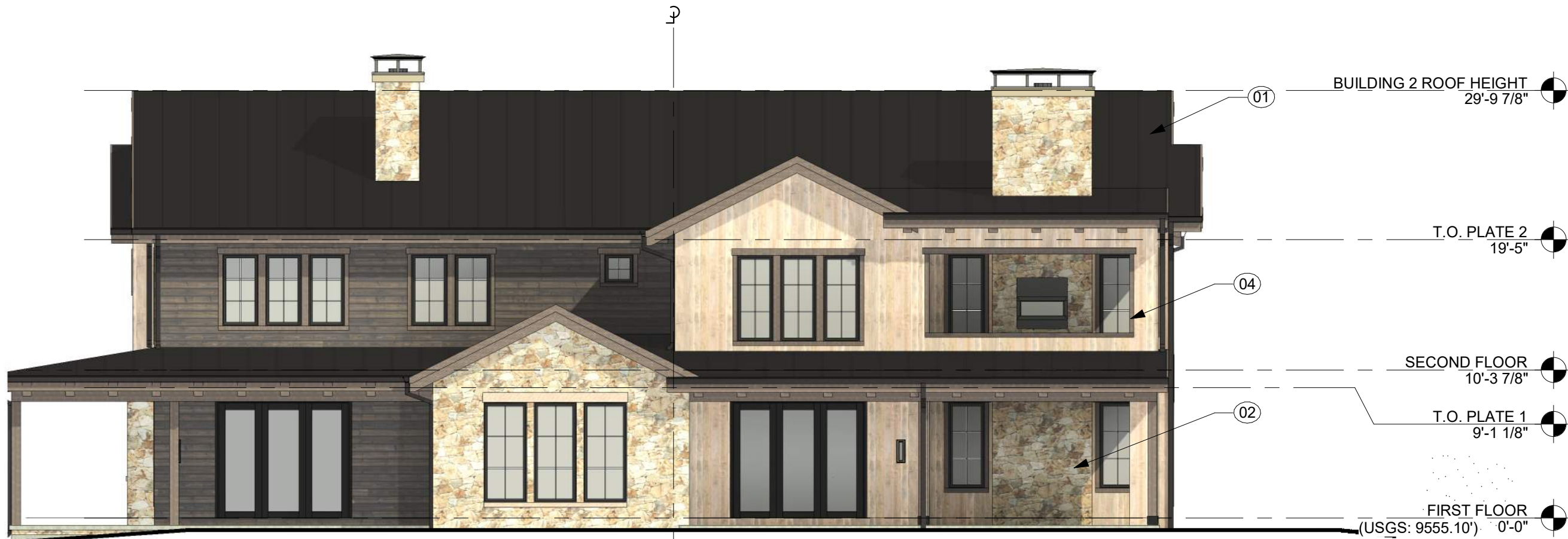
2 BUILDING 2 - REAR ELEVATION A202 SCALE: 1/8" = 1'-0"
