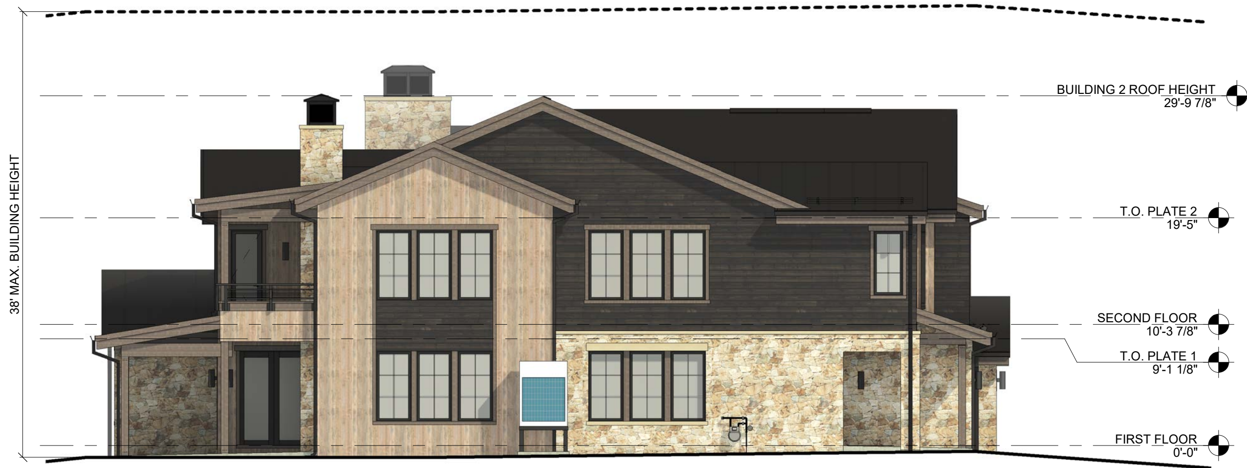
4 BUILDING 2.3 - LEFT ELEVATION - SCHEME 1 A204 SCALE: 1/8" = 1'-0"
