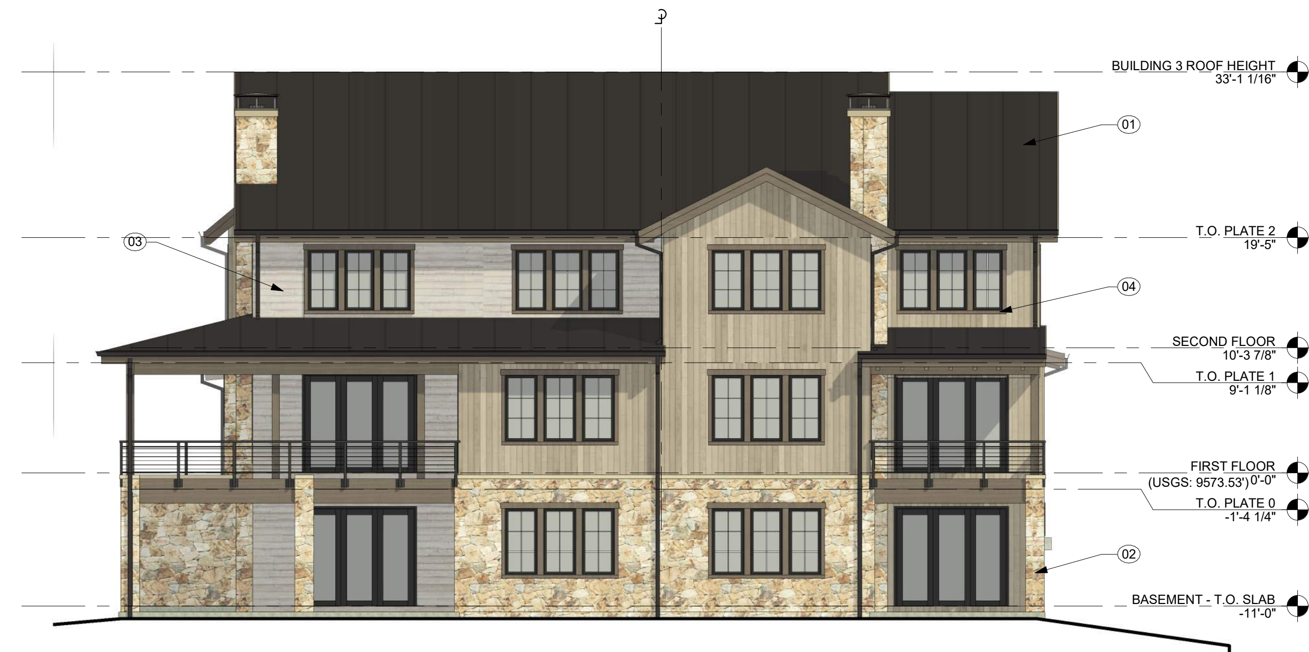
2 BUILDING 3 - REAR ELEVATION A205 SCALE: 1/8" = 1'-0"
