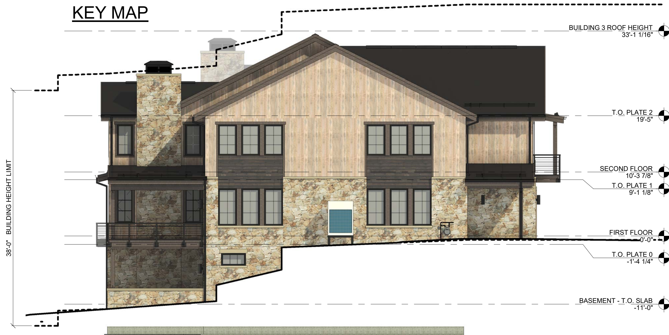
4 BUILDING 3.3 - LEFT ELEVATION - SCHEME 1 A207 SCALE: 1/8" = 1'-0"
