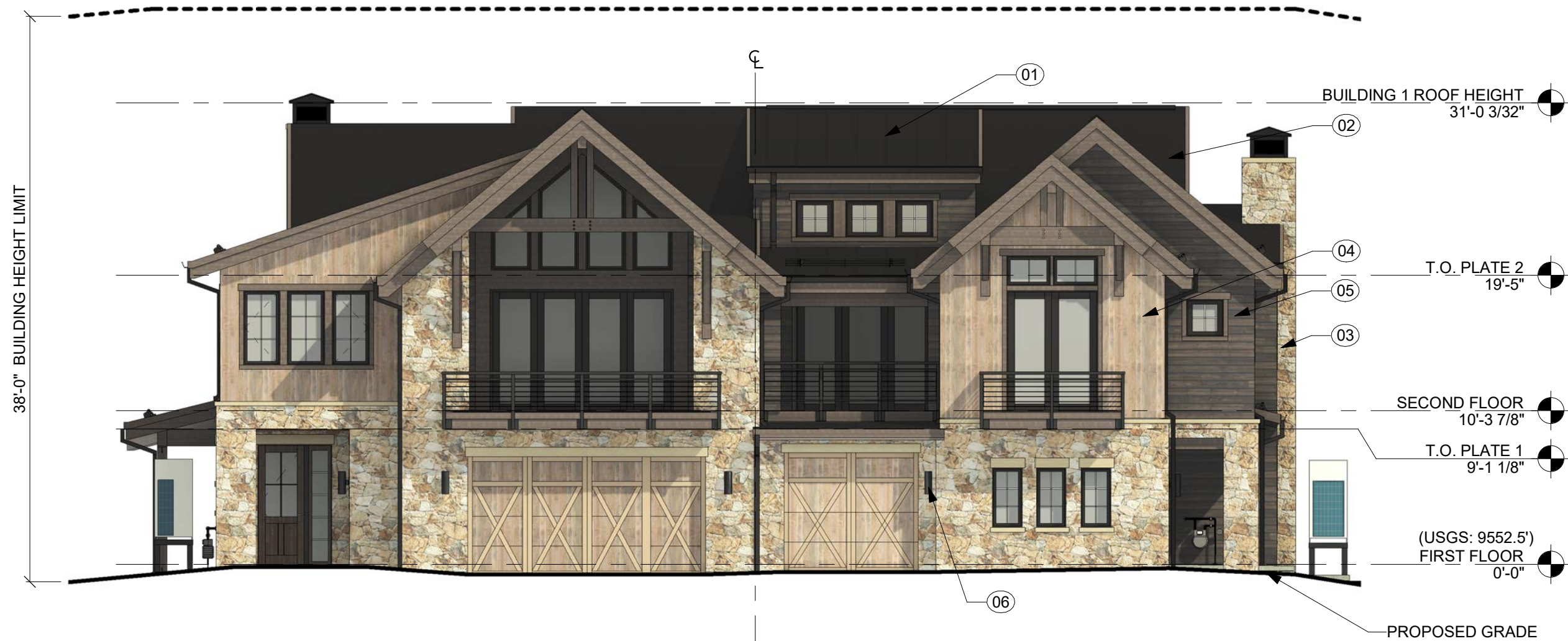
1 BUILDING 1.1 - FRONT ELEVATION - SCHEME 1 A200 SCALE: 1/8" = 1'-0"
