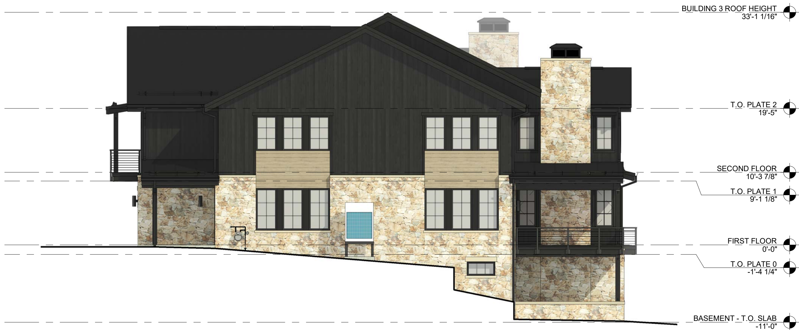
3 BUILDING 3.1 - RIGHT ELEVATION - SCHEME 3 A205 SCALE: 1/8" = 1'-0"
