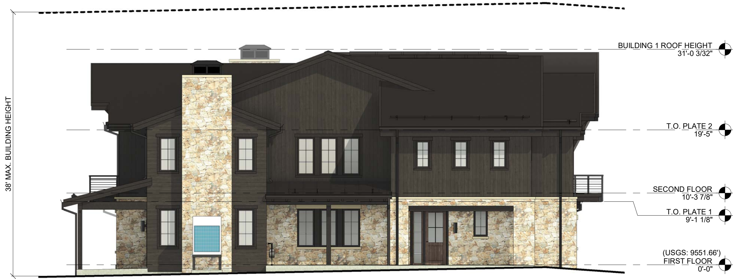
4 BUILDING 1.2 - LEFT ELEVATION - SCHEME 2 A201 SCALE: 1/8" = 1'-0"
