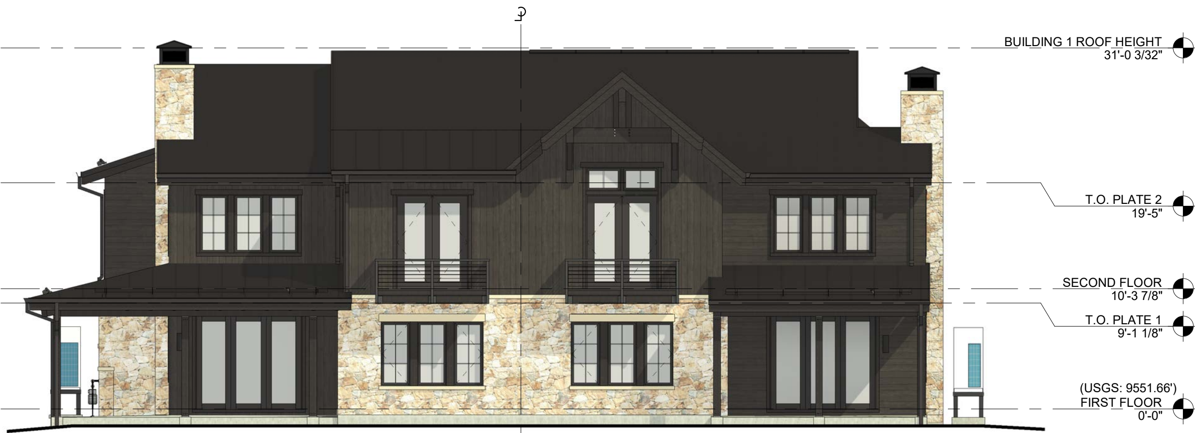
2 BUILDING 1.2 - REAR ELEVATION - SCHEME 2 A201 SCALE: 1/8" = 1'-0"
