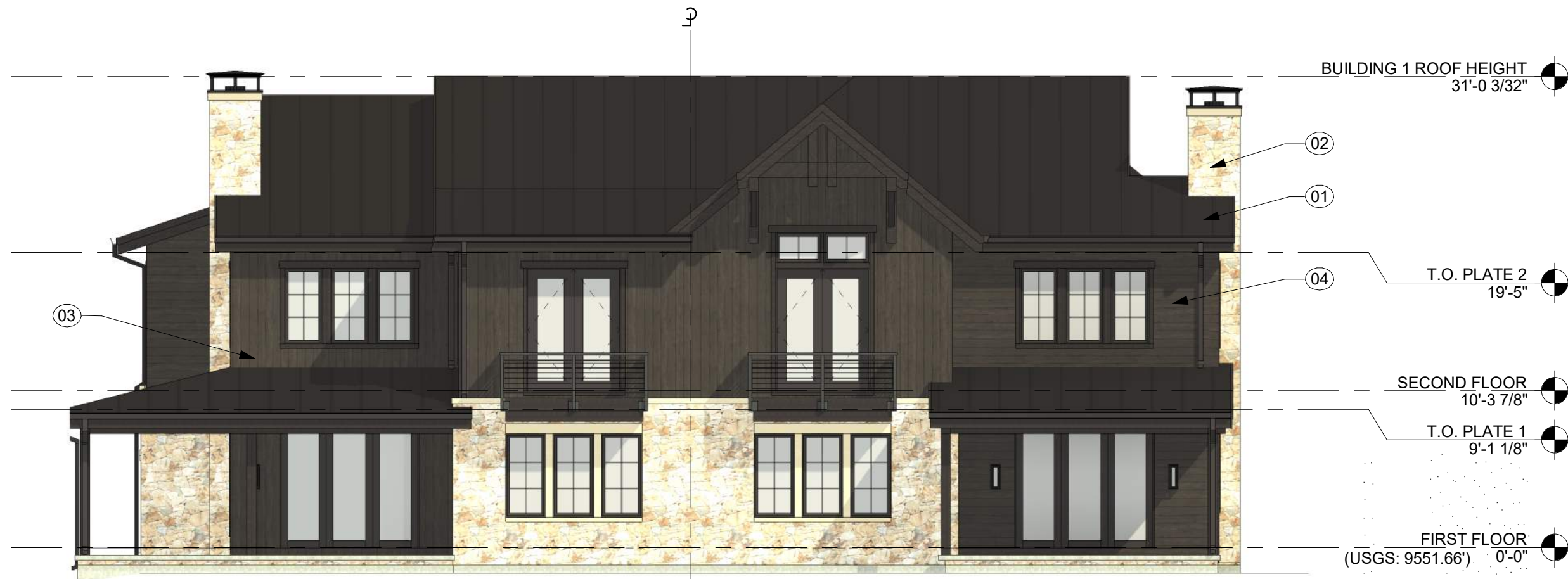
2 BUILDING 1 - REAR ELEVATION - SCHEME 2 A201 SCALE: 1/8" = 1'-0"
