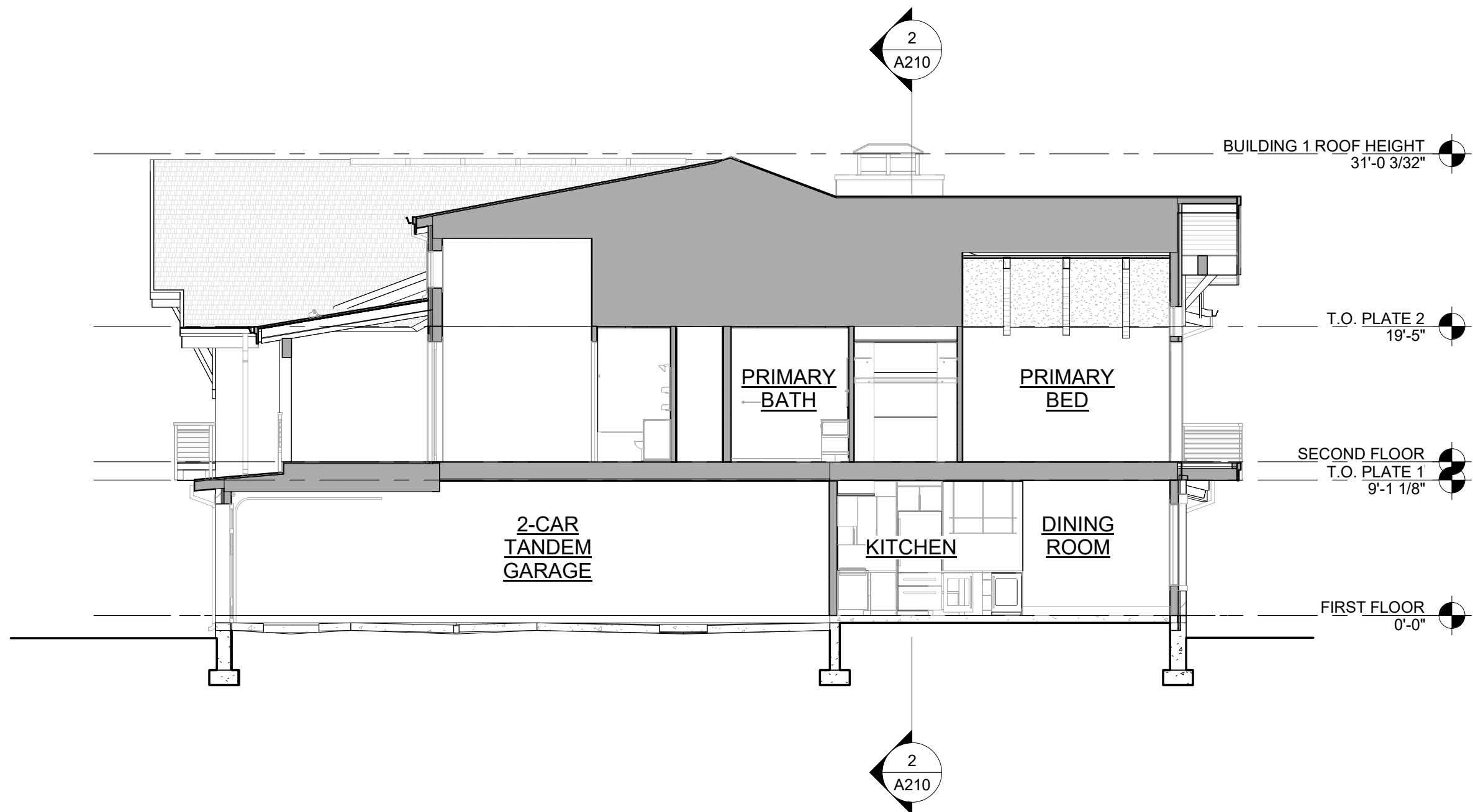
1 A210 BUILDING 1 - SECTION 1 SCALE: 1/8" = 1'-0"
