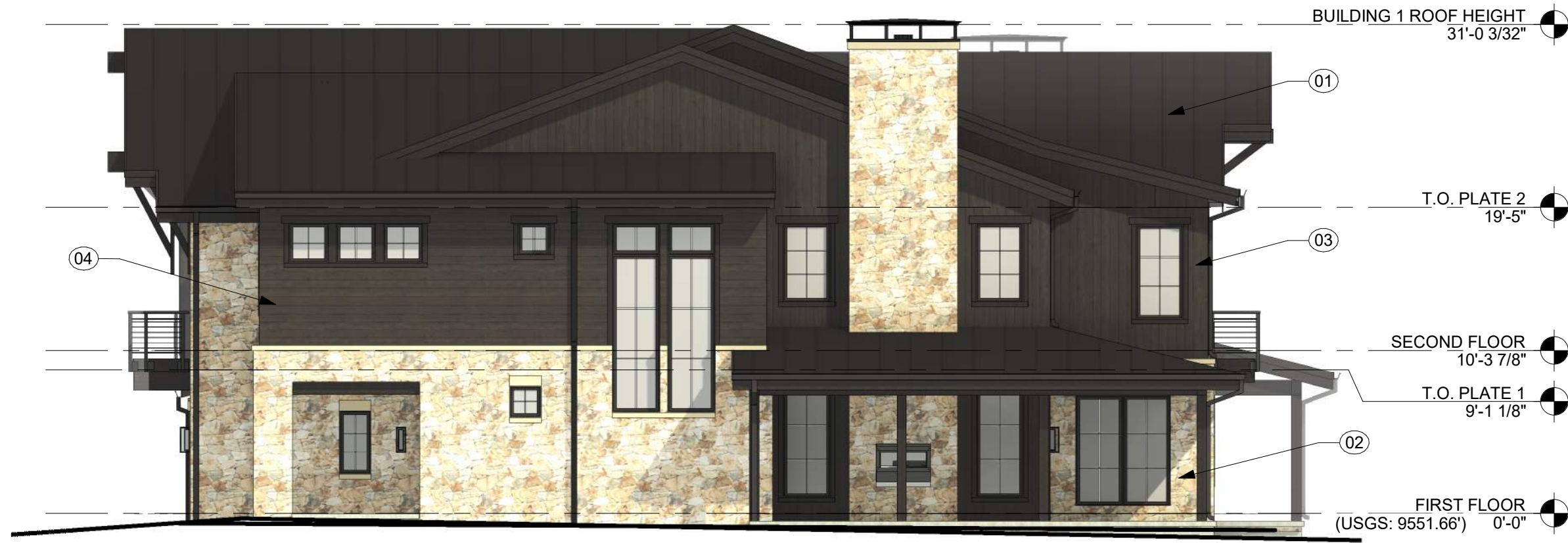
3 BUILDING 1 - RIGHT ELEVATION - SCHEME 2 A201 SCALE: 1/8" = 1'-0"
