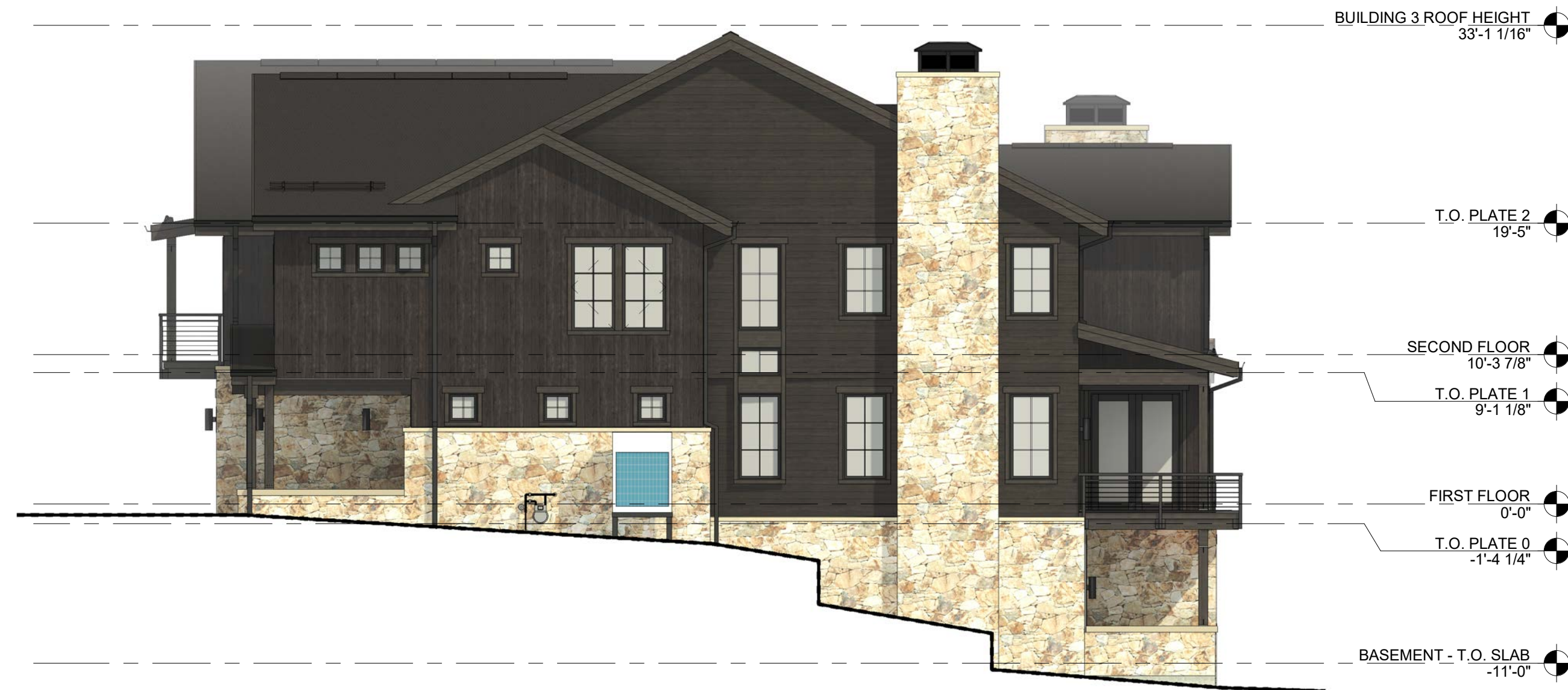
3 A206 BUILDING 3.2 - RIGHT ELEVATION - SCHEME 2 SCALE: 1/8" = 1'-0"
