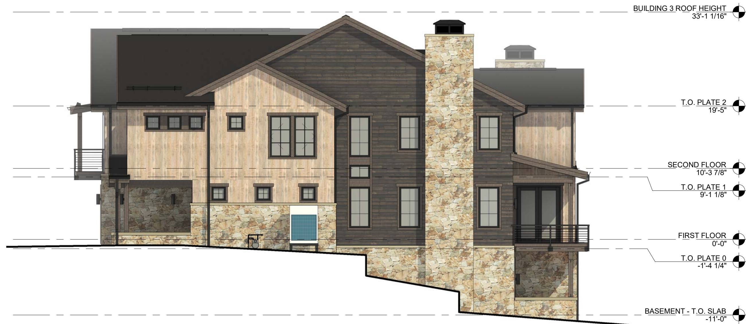
3 BUILDING 3.3 - RIGHT ELEVATION - SCHEME 1 A207 SCALE: 1/8" = 1'-0"
