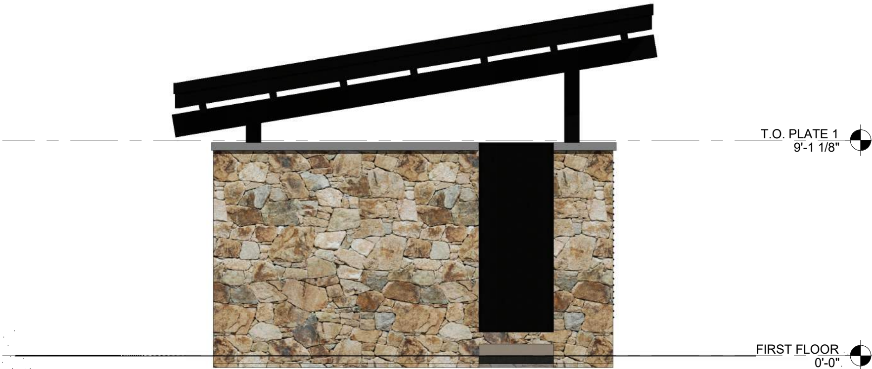
5 TRASH ENCLOSURE - LEFT ELEVATION SCALE: 1/4" = 1'-0"
