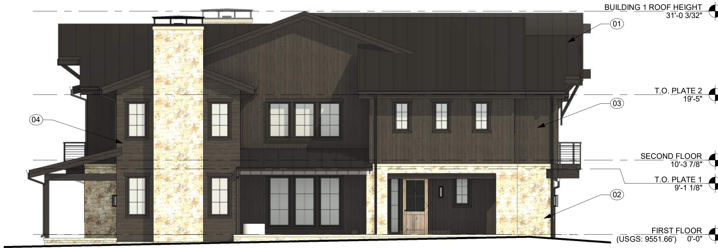
4 BUILDING 1 - LEFT ELEVATION - SCHEME 2 A201 SCALE: 1/8" = 1'-0"
