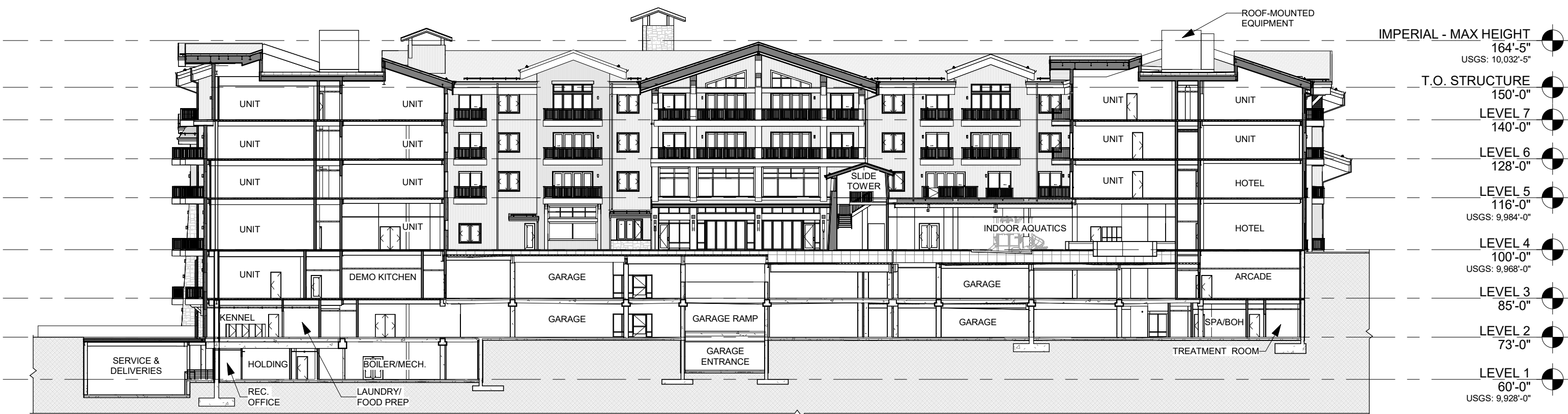
1 A300 BUILDING SECTION SCALE: 1" = 30'-0"
